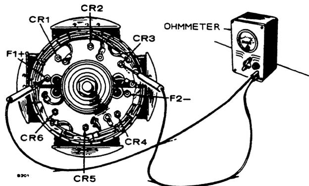
FIGURE 9. TESTING ROTATING RECTIFIERS
