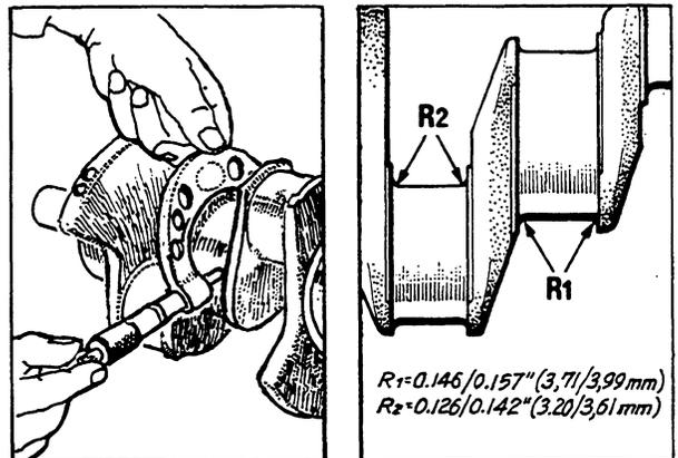
Crank pin standard diameter
