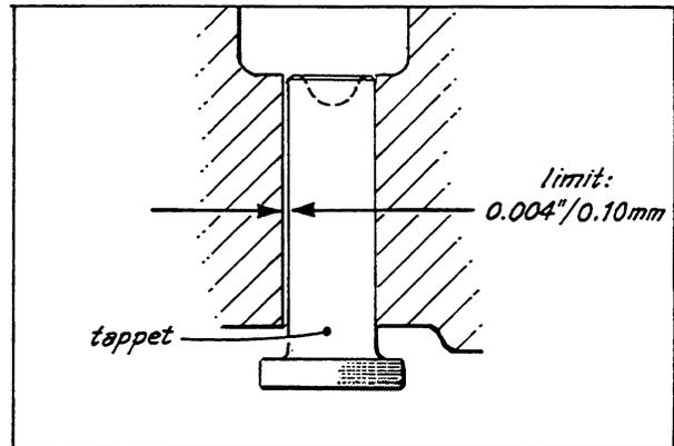
2. Inspecting clearance between tappet and tappet bore
