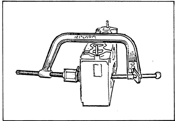
35. Remove each valve from the cylinder head assembly. Use appropriate valve spring compressor to aid in disassembly. Arrange or label valves so as to replace them in the cylinder and guide from which they were removed.
