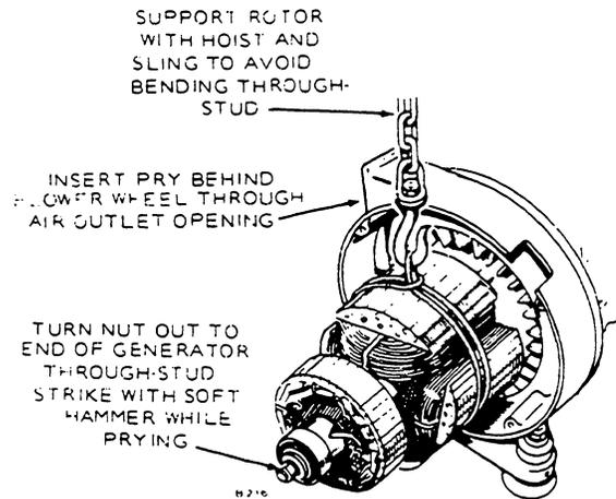
FIGURE 21. ROTOR REMOVAL
