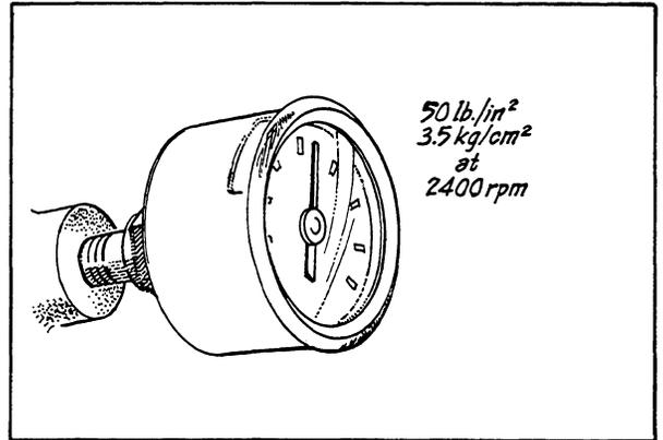
Oil pressure: 3.5 kg/cm<sup>2</sup> (50 lb/in<sup>2</sup>) or more at 2400 RPM
