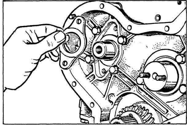
9. Installation of the crankshaft
