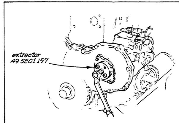
20. Remove the front crankshaft pulley attachment bolt with the aid of a 38 mm socket and draw the pulley off the front crankshaft.
