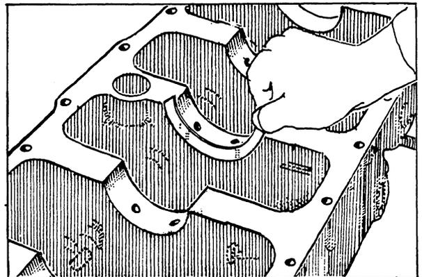
(d) Fit the thrustwasher to the main bearing cap so that the oil grooves on thrustwasher face to crankshaft side. Then install the main bearing cap to the cylinder block with arrow mark of the main bearing cap facing the crankshaft pulley side.
