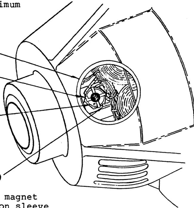
1. Remove the hole cover (item 10) on top anti-drive end of the alternator.
