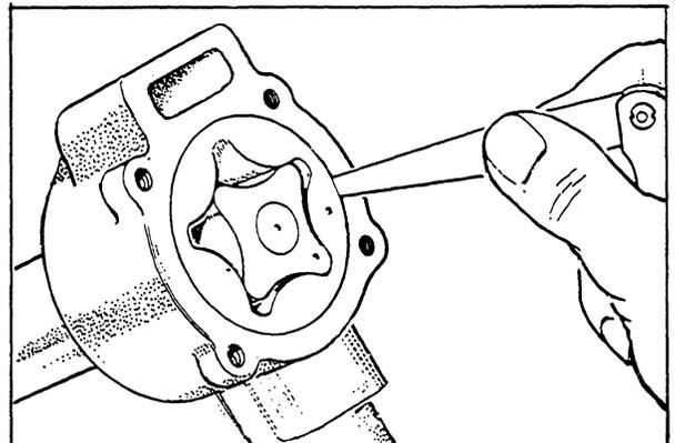
4. Clearance between outer rotor and pump body
