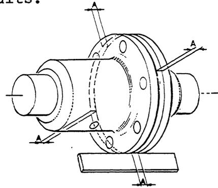
The engine alignment should be rechecked after the boat has been in service for one to three weeks and, if necessary, the alignment remade. It will usually be found that the engine is no longer in alignment. This is not because the work was improperly done at first but because the boat has taken some time to take its final shape, and the engine bed and engine stringers have probably absorbed some moisture. It may even be necessary to re-align at a further period.
