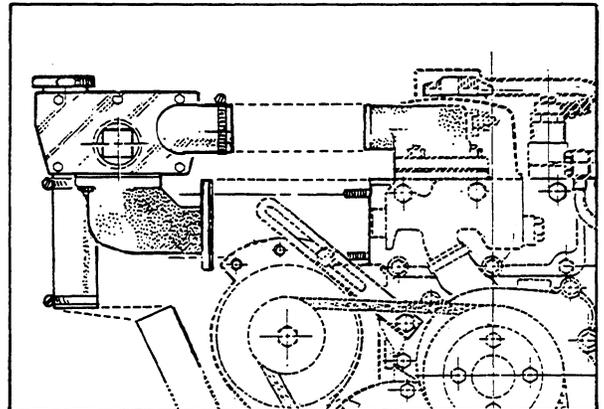
8. Remove the engine alternator and sea water pump.
