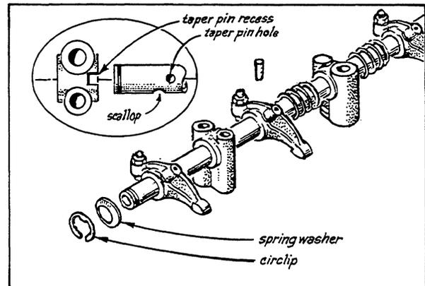
2. Assemble the rocker arm shaft, rocker shaft brackets and rocker arms. Note that the front end of the rocker shaft is identified by a pin protruding from the top and a larger oil hole between the supply holes serving #1 and 2 rocker arms. This pin fits a slot in the #1 rocker shaft support which prevents the shaft from turning and cutting off the lube oil to the rocker arms and valves.
