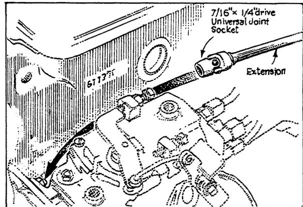
(d) Mount the injection pump on the gear case, then tighten the pump drive gear attaching nuts.
