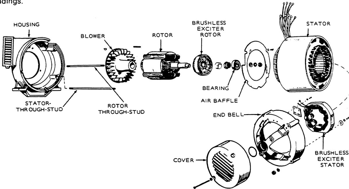
FIGURE 20. GENERATOR DISASSEMBLY
