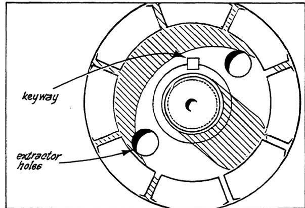
(e) With the use of extractor #49 SE01 157 apply sufficient pressure to loosen the pump from the keyed gear. The loose hold down nuts will prevent the pump from falling from the engine.
