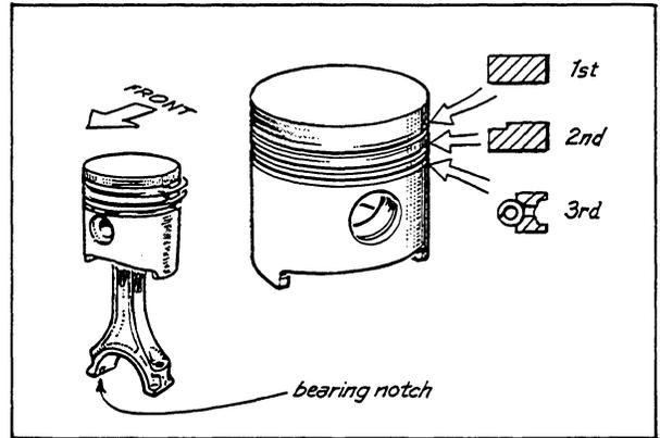
(c) Install the piston rings to ring grooves on the piston with the inscription mark on ring upward.
