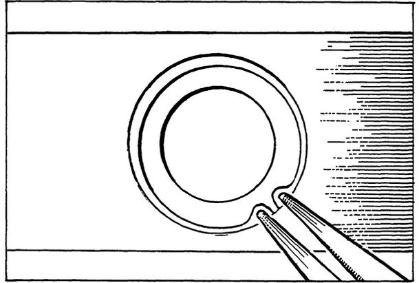
Note: If the piston pin is tightly fitted, heat the piston head with the aid of a hot plate or similar device.
